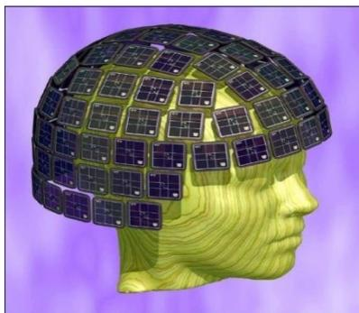
1 magnetometer and 2 planar gradiometers at each location
