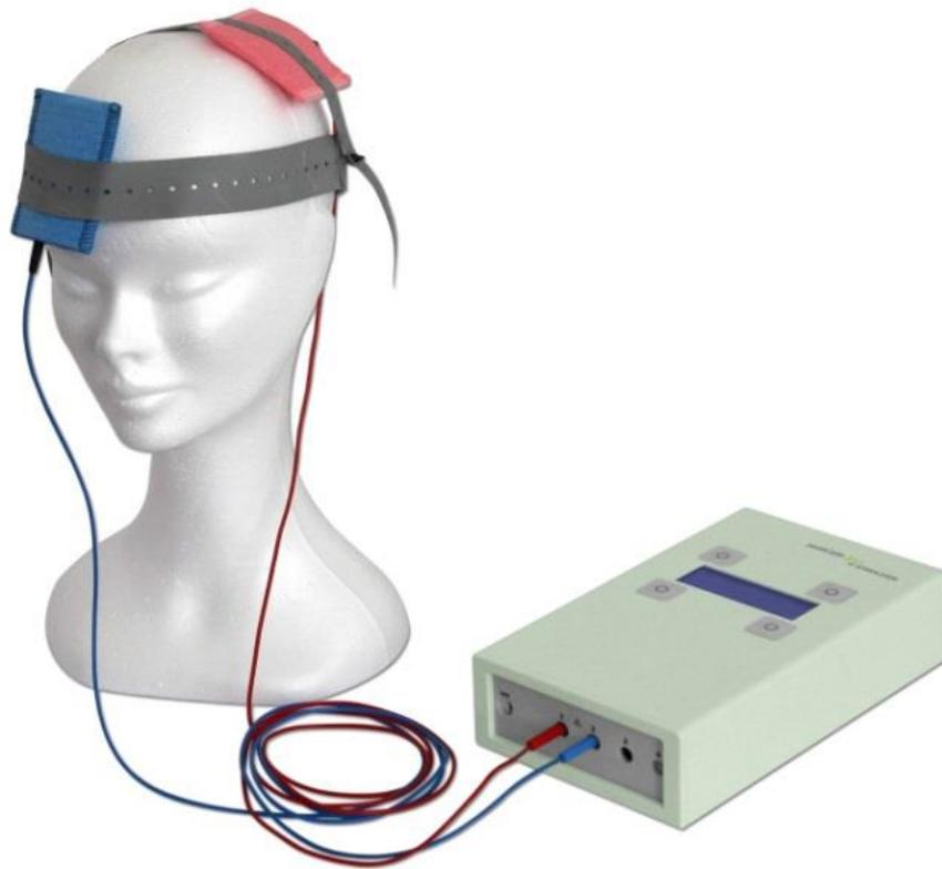
A small electrical current (0.5-2 mA) is passed between two electrodes placed on the scalp
