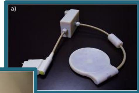
The MR coil array is placed between the TMS and head of the participant
